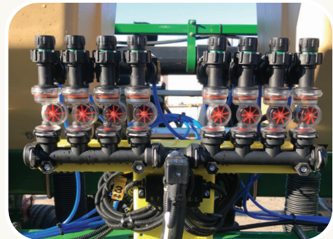
EFM systems are developed by OEM manufacturers using WILGER parts
